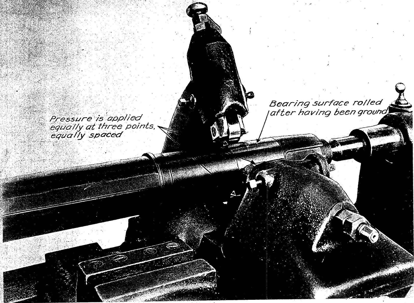
Armature Construction, Rolling The Bearing Surfaces of Armature Shafts For Railway Motors
